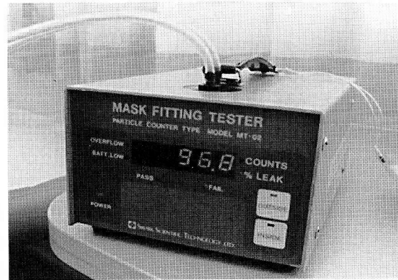
Fig. 1 The outside appearance of the Mask Fitting Tester Model MT-02 TM , Roken type
